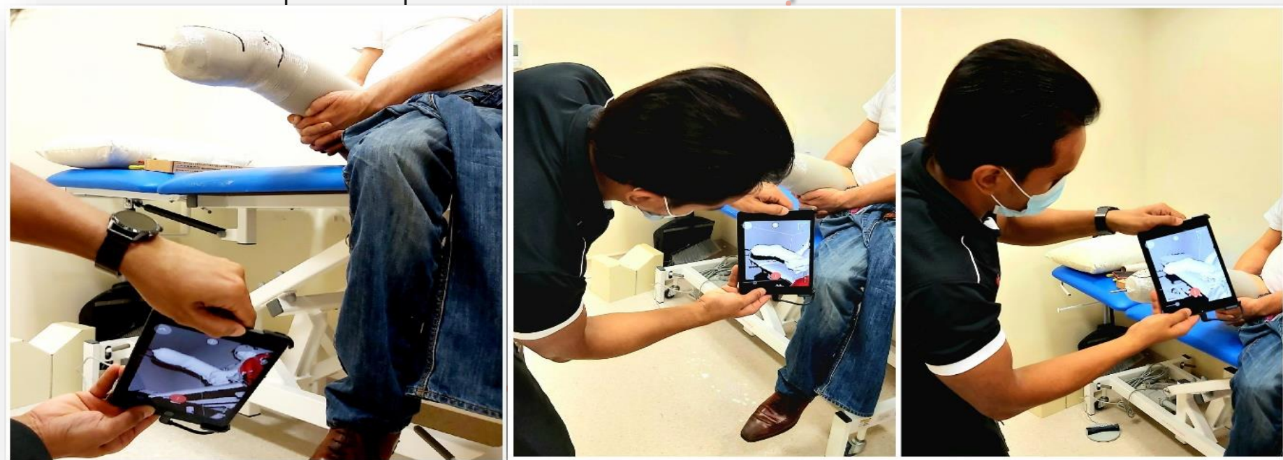
Technician performing a 3D scan of a transtibial amputee's stump using a handheld scanner
