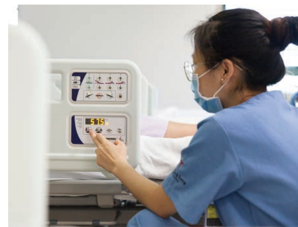
New hospital beds are equipped with a weighing scale, and a fifth wheel to cut down manpower and operational time.
