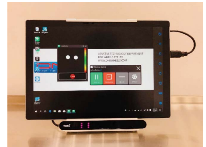
Figure 1. Tobii – calibration of the eye gaze tracker device. The Tobii eye gaze device is connected to the tablet. On the screen, the two white dots indicate the detection of the user's eyes.
